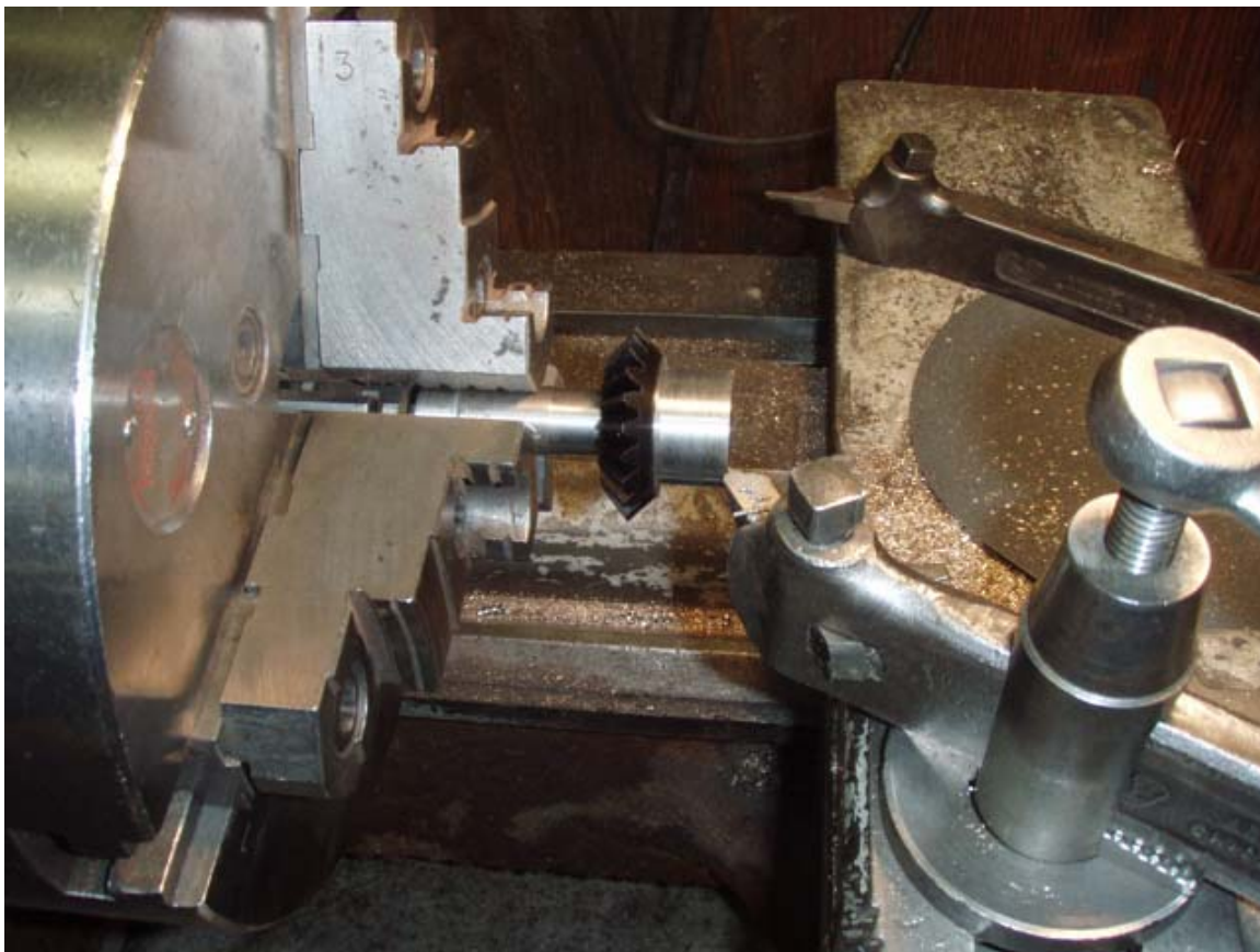
Figure 2 - Machining Gear Hub, note use of mandrel to hold gear
