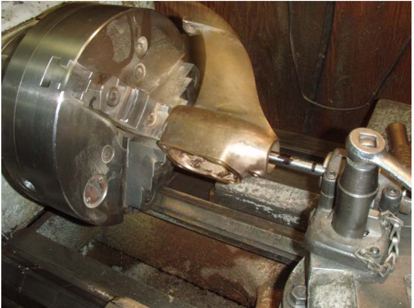
Figure 1 - Boring gear housing in the lathe
