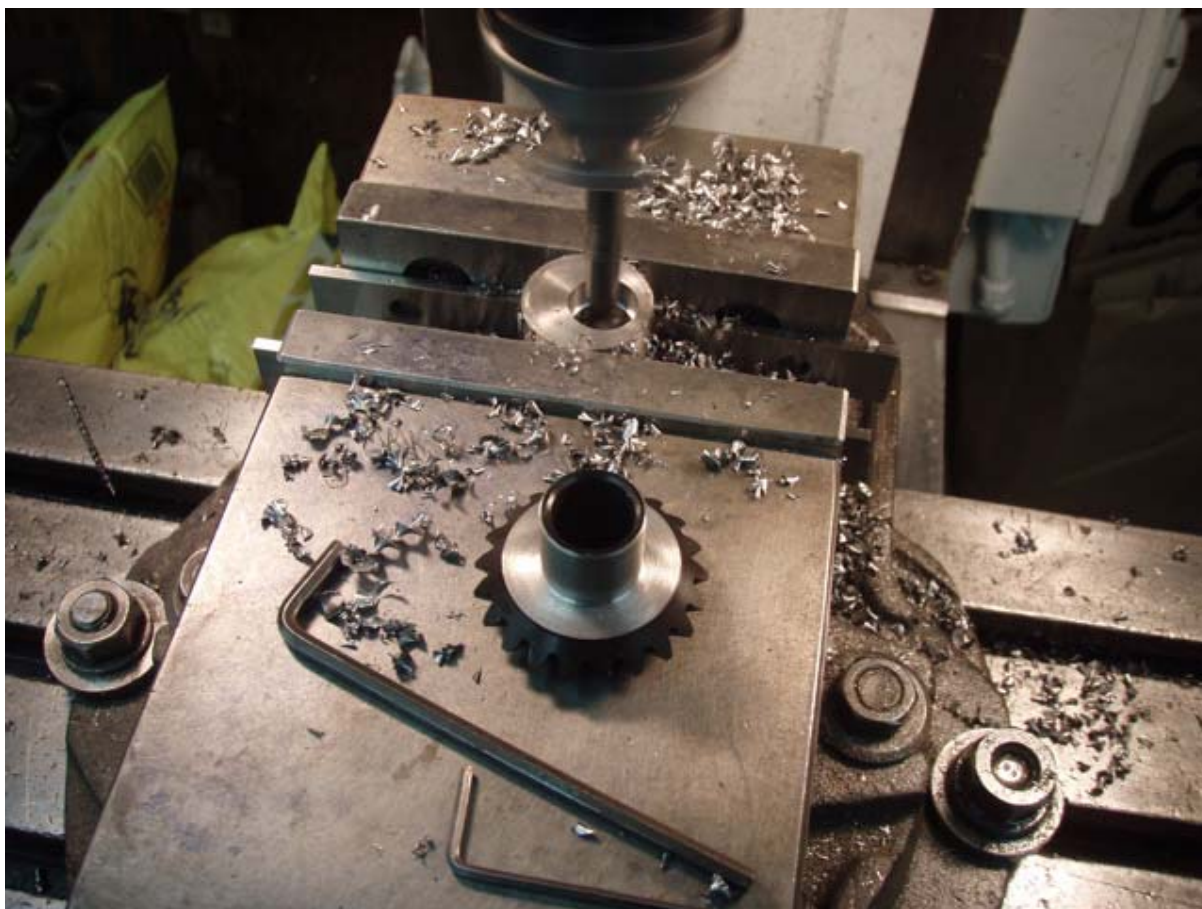
Figure 3 - Machining the off-set hole in the pump cam
