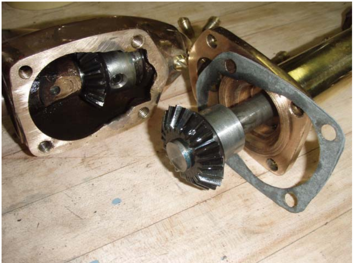
Figure 5 - Gears before final assembly, note amount of driveshaft that protrudes from the bottom of gear
