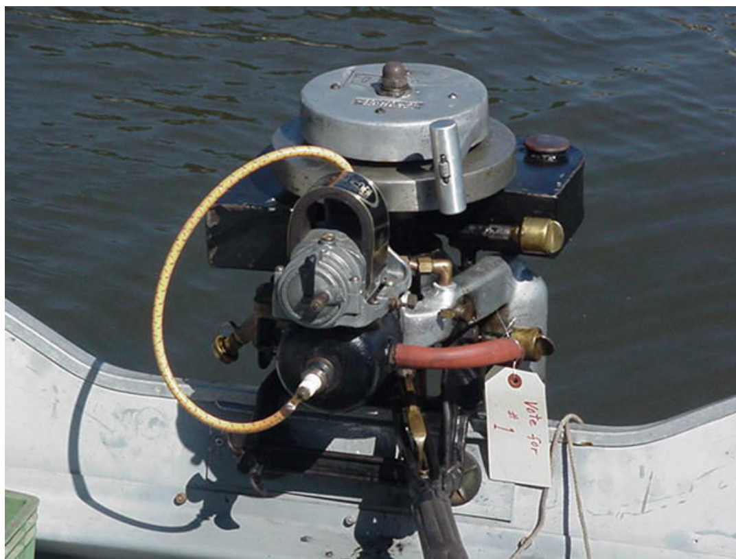
Two Views Of A Caille 5-Speed RBM with gear-driven Bosch Magneto and recoil starter (Owner - Tom Goeprich)
