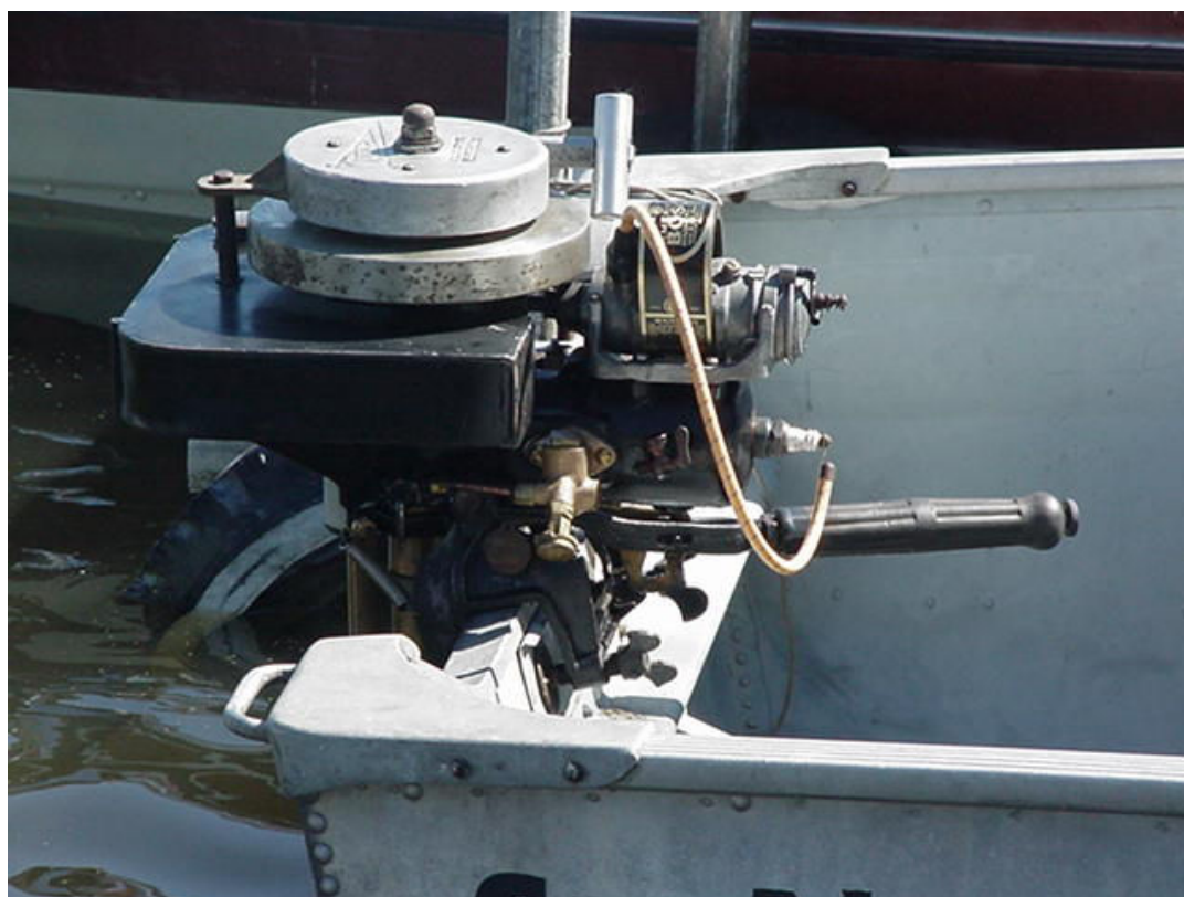
Two Views Of A Caille 5-Speed RBM with gear-driven Bosch Magneto and recoil starter (Owner - Tom Goeprich)
